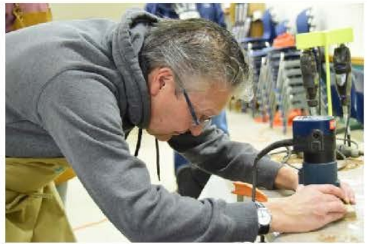
Route out 1/8 th inch deep not quite to the pencil line
