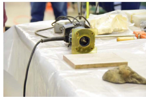
Router ready to remove the bed for the stone.
